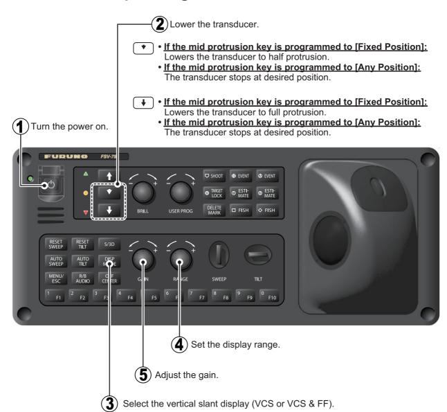
**Note:** In the default setting, slant (S) and vertical Slant (VCS) modes are active. To use other display modes, register the display mode to use from the menu. For how to register display modes, see section 1.6.2.
