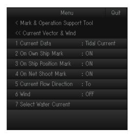
[1 Current Data]: Selects how to display current data, absolute or in relation to current layers (1, 2, 3, 4 or 5).
