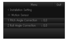
[1 Pitch Angle Correction]: Offsets the pitch angle at the motion sensor.
