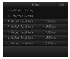
[1 NMEA1 Baud Rate] to [5 NMEA5 Baud Rate]: Set the baud rate for each NMEA port. The choices are [4800bps], [9600bps], [19200bps], [38400bps].
