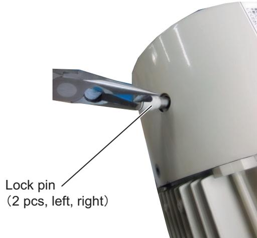
6. Remove the motor brake cover.
