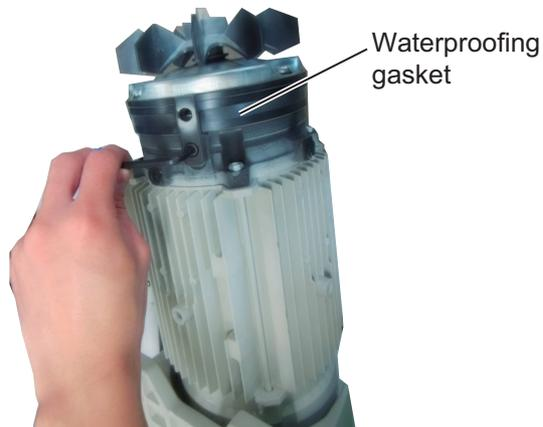
8. Loosen a set screw to remove the fan.
