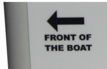
Figure 9. WASSP Sensor Box Alignment
