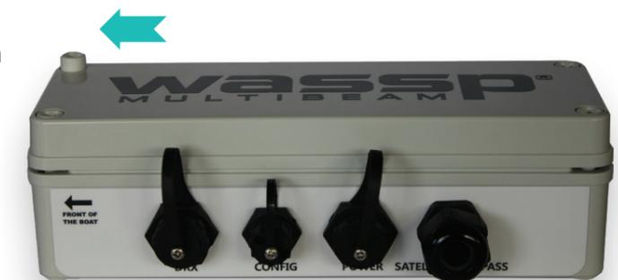
5. Insert the Satellite Compass cable into the box through the gland. Insert the wires into the terminal block seen below and then tighten the terminal screws. See *"Appendix A.3 Satellite Compass Terminal Block"* for Satellite Compass pin out.
