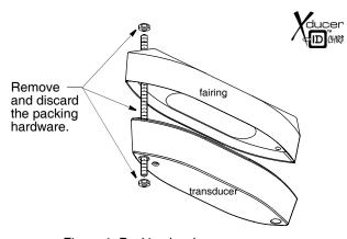
Figure 1. Packing hardware Copyright © 2007 Airmar Technology Corp.
