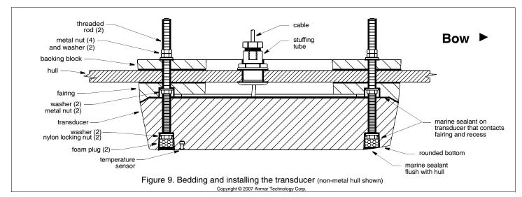
4. Push the *uncolored* section of each threaded rod through the fairing, the hull, and the backing block until the washer rests inside the recess in the fairing (Figure 7). With a person stationed inside the vessel, secure each rod with a washer (bedded side against the backing block) and double stainless steel nuts. Use a wrench to hold the lower nut while tightening the top nut against it.
