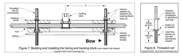
7. The remaining section of the fairing with the cutting guide will be used as the backing block inside the hull. It will provide a level surface for tightening the nuts on the threaded rods.
