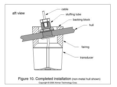
rechecking. If there is a small leak, there may be considerable bilge water accumulation after 24 hours. If a leak is observed, repeat the bedding and installing procedures beginning on page 3 **immediately**.
