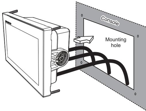
9. Fit the flat washers and nuts to the threaded rods.
