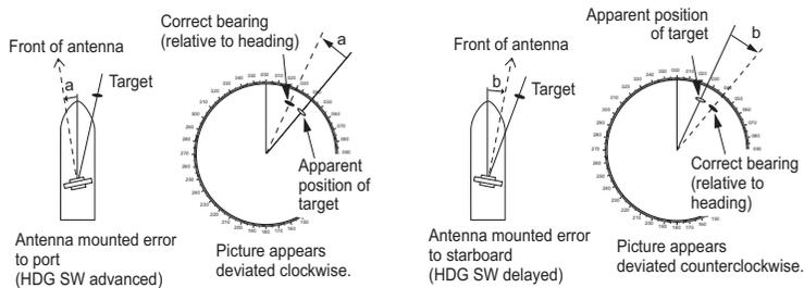
1. Turn the boat towards a target. The target should be oriented directly forward of the bow.
