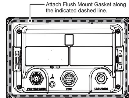
4. Mark and cut the installation hole, then drill four bolt holes, referring to the Flush Mount Template at the back of this manual.
