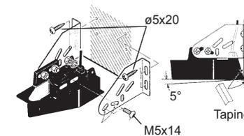
5. Fill the gap between the wedge front of the transducer and transom with epoxy material to eliminate any air spaces.
