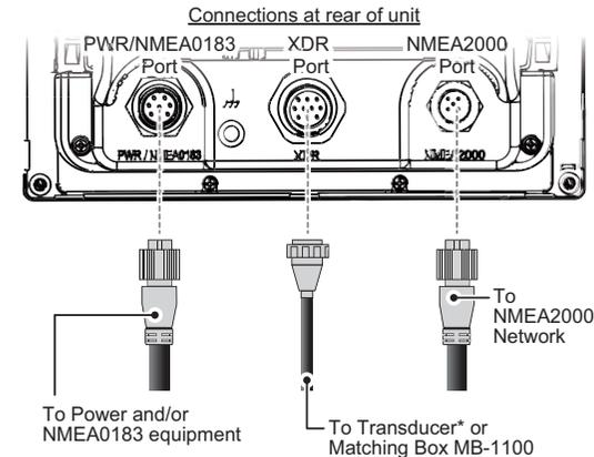
**Note:** Do not connect/disconnect the cables connected to the unit while the power is turned on. The unit may be damaged.
