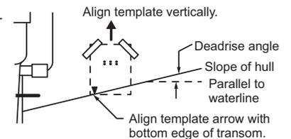
**Fiberglass hull:** Minimize surface cracking by chamfering the gelcoat. If a chamfer bit or countersink bit is not available, start drilling with a 6mm or 1/4" bit to a depth of 1 mm (1/16").
