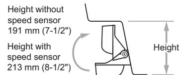
**Note 2:** Avoid mounting the sensor where the boat may be supported during trailering, launching, hauling, and storage.
