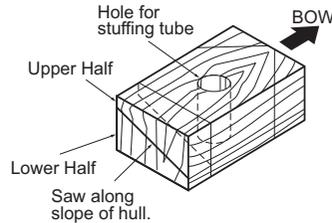
3. Drill a hole just large enough to pass the threaded stuffing tube of the transducer through the hull, making sure it is drilled vertically.
