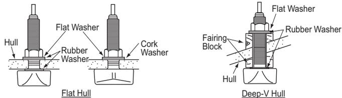
**Note:** Do not over-stress the stuffing tube and locknut through excessive tightening, since the wood block will swell when the boat is placed in the water. It is suggested that the nut be tightened lightly at installation and re-tightened several days after the boat has been launched.
