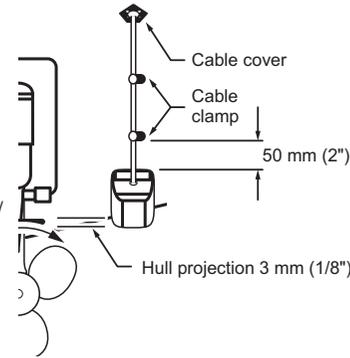
**How to attach the sensor to the bracket**
