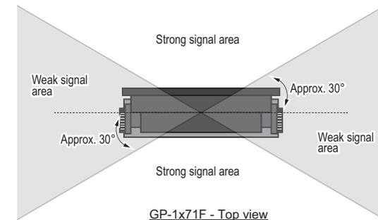
The unit should be located within the following distances from the radar sensor, to ensure a stable connection.
