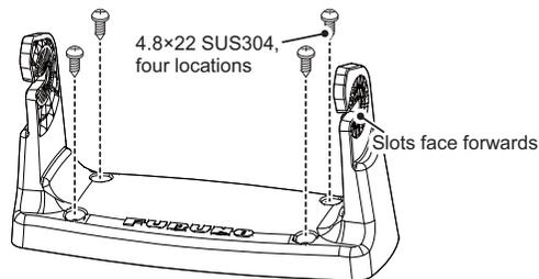
4. Loosely fasten the knob bolts, removed at step 1, to the Display Unit. Leave approximately 10 mm of thread exposed.
