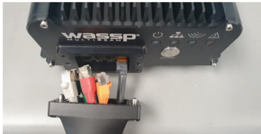
4. Adjust the cable cover to mate with DRX front panel by aligning both dowel pins, then insert & tighten the 4 Hex screws.
