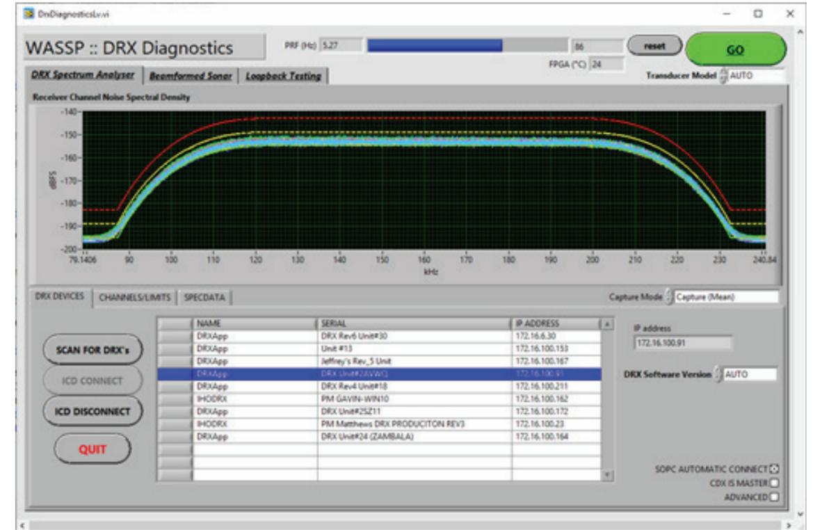
All 26 Channels should show very similar levels. If any channel (or likely set of four channels) show as low, recheck the RJ45 connections to the DRX front panel.
