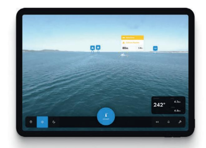
The OSCAR system feeds into your chart plotter, on-board computer, tablet or smartphone. The user interface displays a choice of three viewing modes: low light augmented reality view, thermal augmented reality view and map view.
