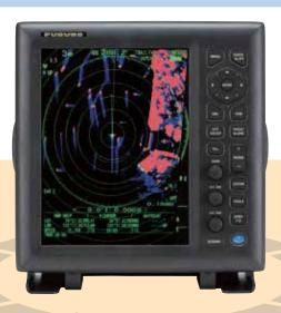
**Radar FR-8xx5 series** When interfacing with FR-8xx5 series, AIS interface IF-1500AIS is needed. AIS target
