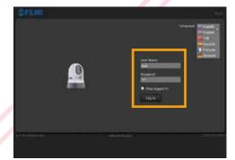
M100 / M200 Series cameras support DHCP and UPnP to simplify the process of finding the camera on your network, and connecting to it using a Web browser.
