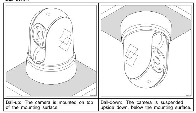
The default video image orientation is for the ball-up configuration; if the camera is to be mounted in the ball-down configuration then the video image must be rotated. To rotate the video image, you must either:
