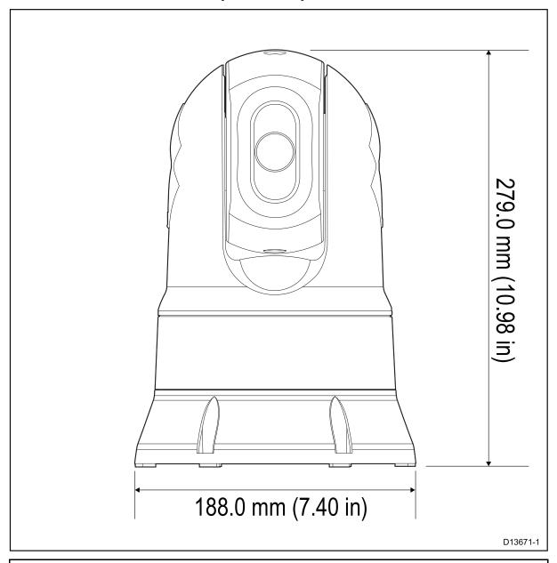
Note: Base diameter with riser base-seal fitted is 190 mm (7.48 in).
