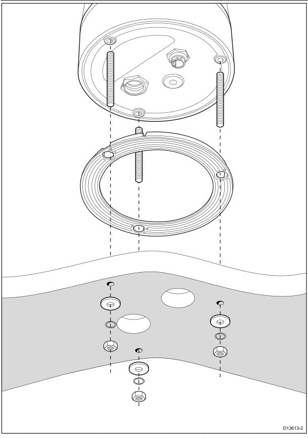
1. Using the template supplied, mark and drill the holes for mounting the camera.
