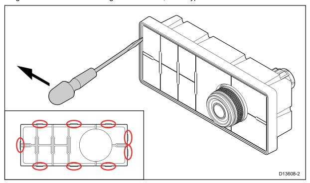
**Tip** To help prevent scratching the product, cover the tip of your screwdriver blade with a small piece of insulation tape.
