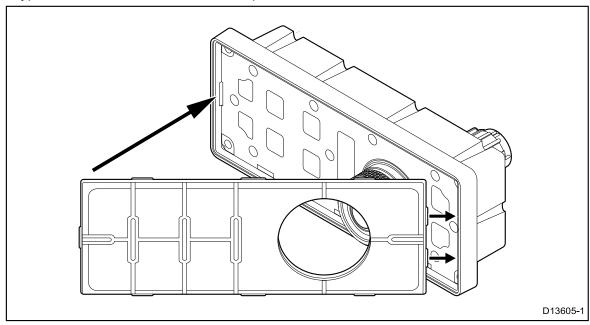
3. Close the opposite end of the keypad mat into the keypad, ensuring that the tab slides into the notch provided. Push all of the tabs on the longer sides into their notches (you should hear a click as each tab engages).
