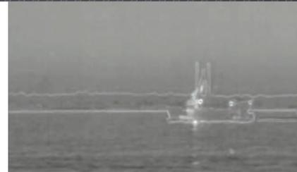
Exclusive FLIR Multi-spectral Dynamic Imaging (MSX) technology enhances thermal images with edges, patterns, text, and other high-contrast elements not always visible to the thermal camera alone.
